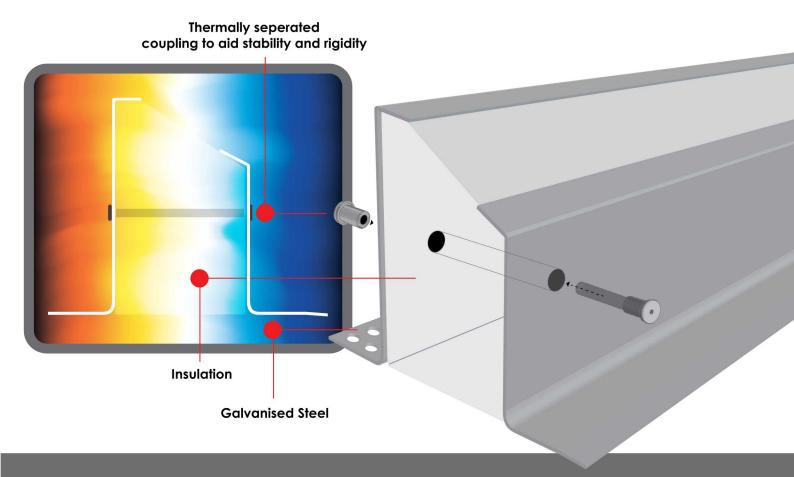
Improving the Thermal performance of walls is crucial for energy efficiency in buildings and addressing thermal bridges like Lintels, is a key aspect of this and will achieve better psi values.
